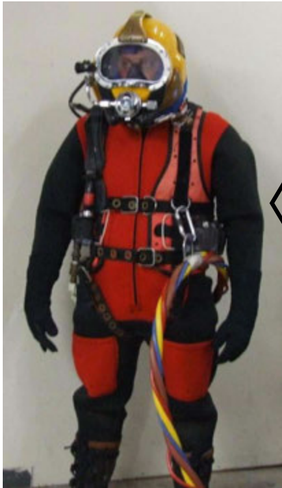
Carabineer Securing Umbilical, Diver's Left Chest: -Secured to upper D-ring at Divers left side, leading under left arm and under emergency cylinder at back.
