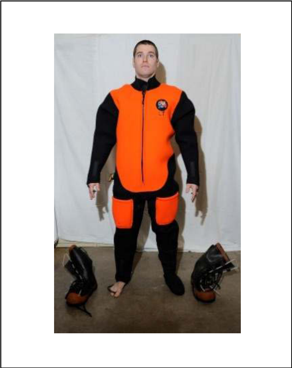
Figure 4-3-1 Hot Water Suit
