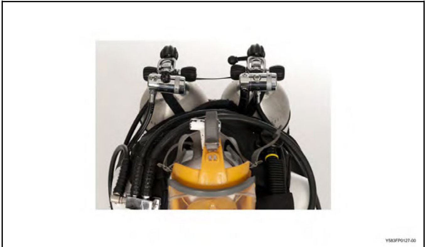
Figure 5B-4 Two Single 2265-Litre (80-Cubic Foot) Cylinders Rigged for CABA Ice Diving with Mini Gauge
